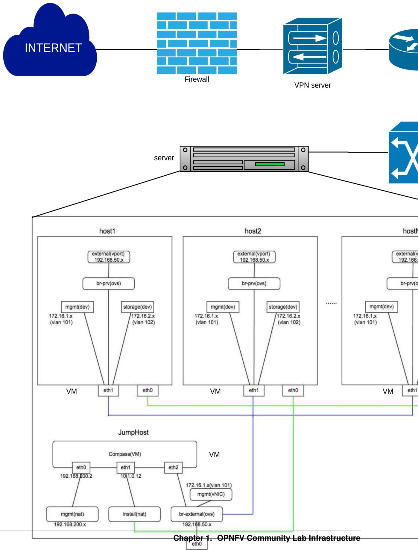
Figure 3: virtual deployment pod network configuration
