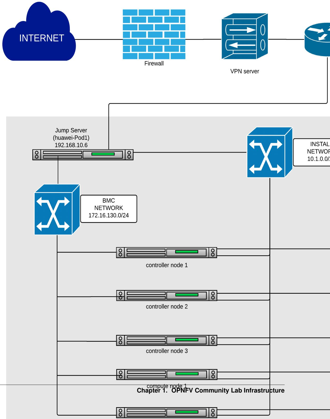
Figure 1: Huawei lab pod1 topology
