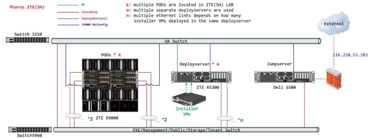
All the PODs share the same **Jump Host** for only one public IP address is allocated for ZTE Pharos Lab. Deploy servers are separated from Jump Host. Each POD has its own **Deploy Server**.
