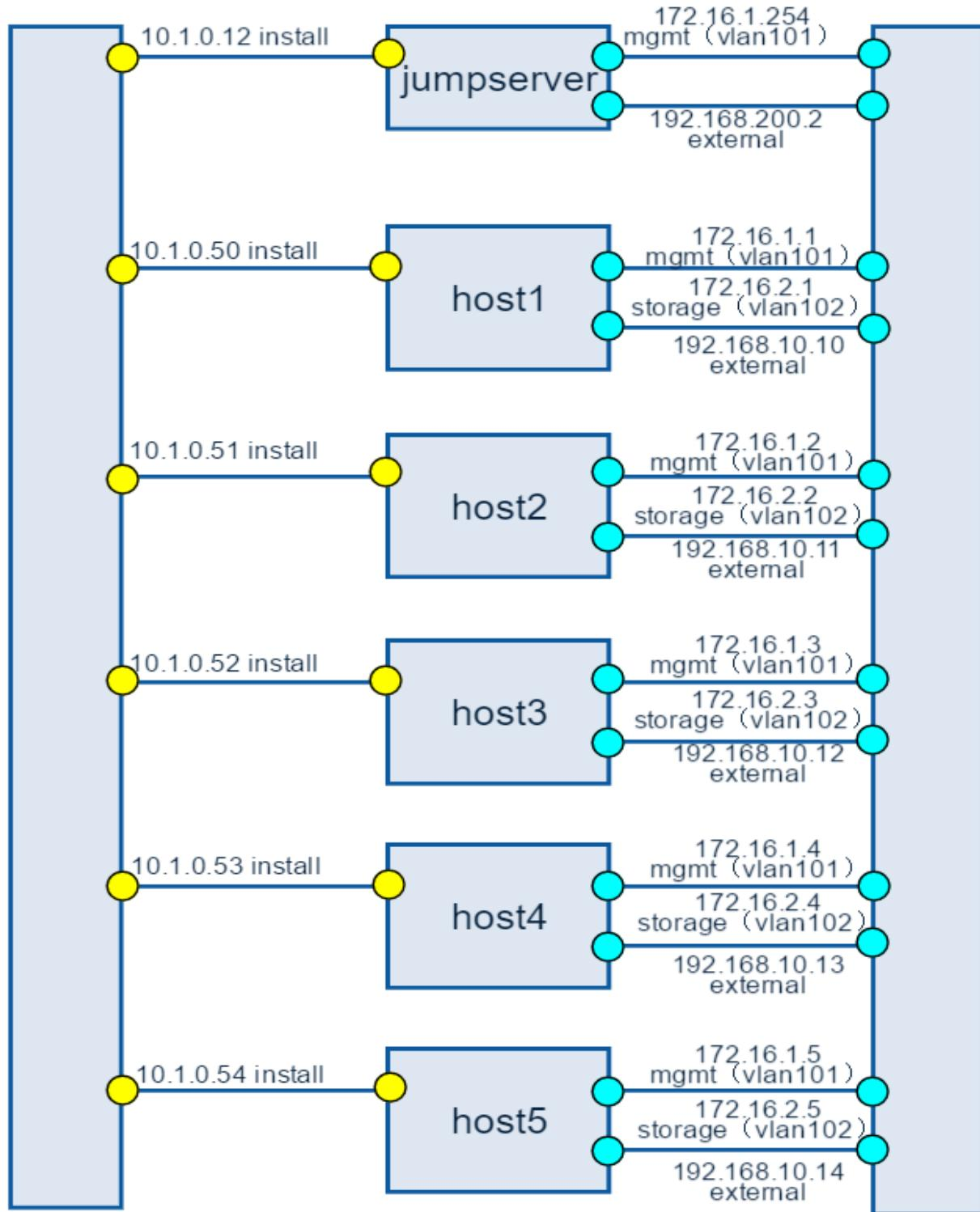
Figure 2: Full Pod network configuration
